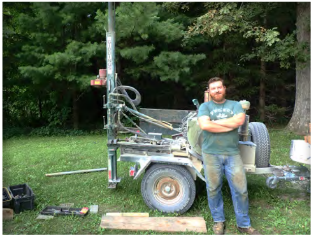
MS student and IGS staff member Phil Kerr using a Giddings soil probe to collect Quaternary cores for his research on the Iowan Erosion surface and Middle Wisconsin Glaciation
