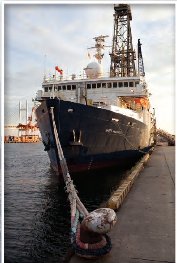
The JOIDES Resolution is a research vessel that drills into the ocean floor to collect and study core samples. It is funded by the National Science Foundation and an international consortium.
